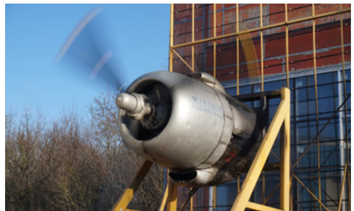
Fig. 4 Prop engine at Wintech façade testing facility
