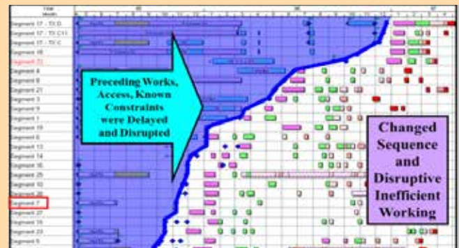
The as-built programme of the segments of the runway and taxiways hard-core (pink and green) and tarmac (dotted and solid red) layers
